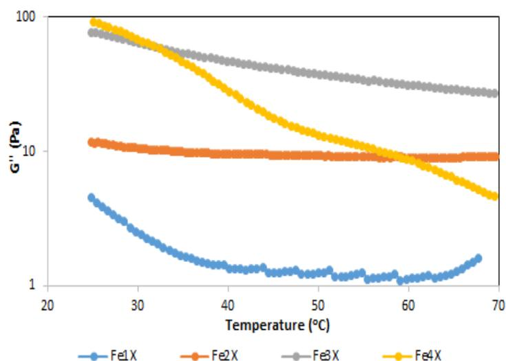
**Figure 2:** Pectin- $Fe^{2+}$  temperature sweep curves for Loss modulus ( $G''$ ) with LMH pectin.
