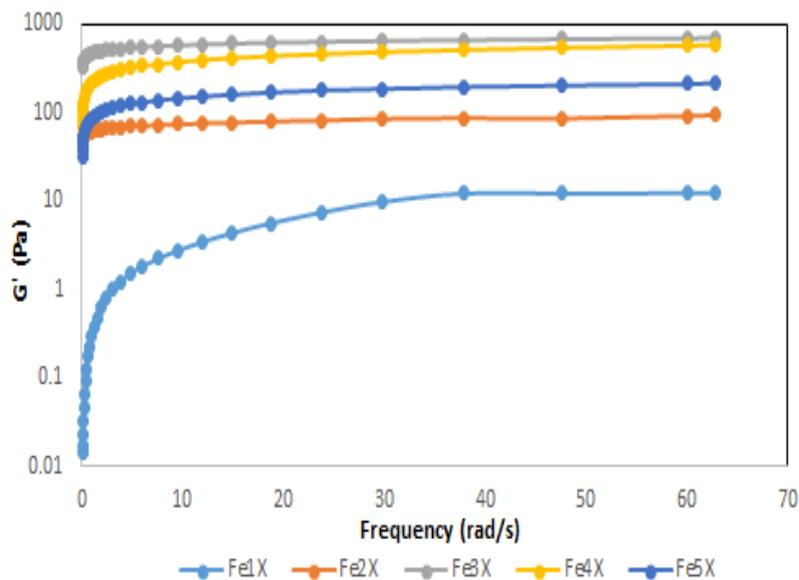
**Figure 3:** Pectin-Fe<sup>2+</sup> frequency sweep curves for Storage modulus (G') with LMH pectin.
