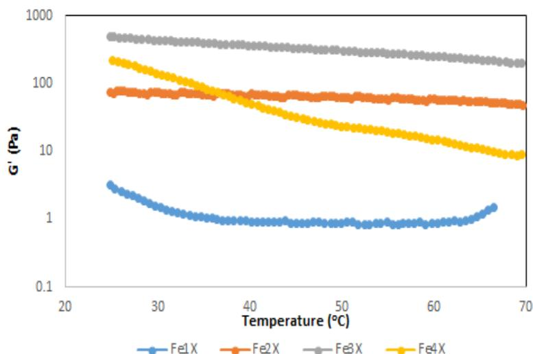
**Figure 1:** Pectin- $Fe^{2+}$  temperature sweep curves for Storage modulus ( $G'$ ) with LMH pectin.
