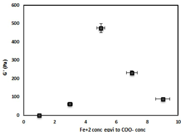
**Figure 5:** Storage modulus (G' corresponds to frequency of 1rad/s in frequency sweep curves) curve for Fe<sup>2+</sup> with using LMH pectin.
