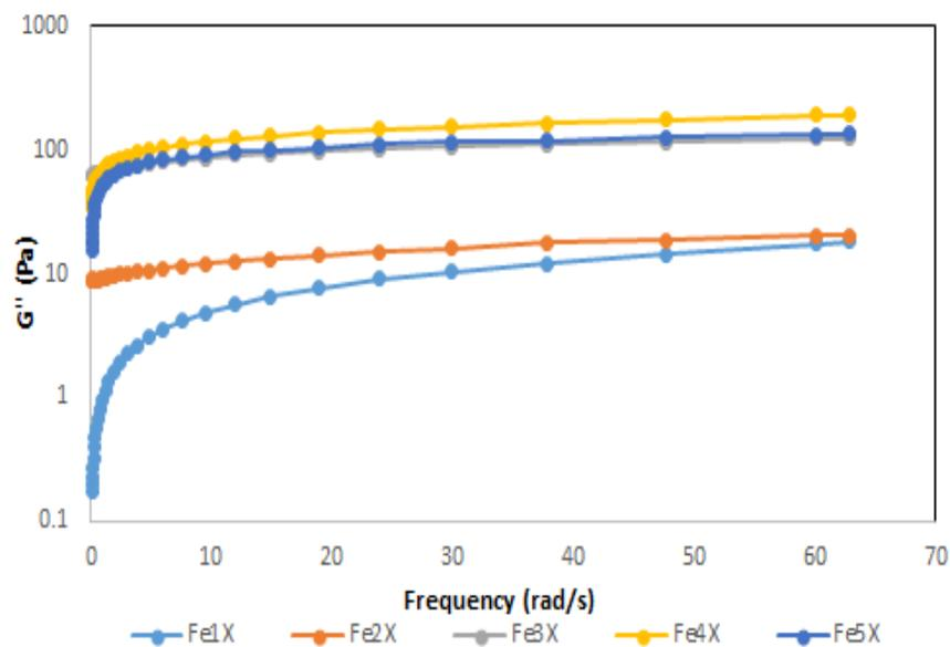
**Figure 4:** Pectin-Fe<sup>2+</sup> frequency sweep curves for Loss modulus (G'') with LMH pectin.
